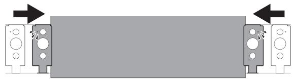
• To print on thin or soft media, swap left and right edge holders and attach them as shown in the figure below so that the hole on the edge holder is located on the inside of the holder. This will hold down wider area on roll media.
