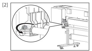
Twist the knob bolt on the **left** side of the media holder anticlockwise to loosen.
