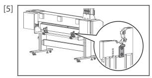
(When looking from the rear side of the printer) Use the screwdriver to loosen two screws securing the roller shaft guide plate to the right media holder.
