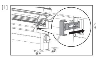
From the front side of the printer, push the media feed lever to hold the media flat with pressure rollers.
