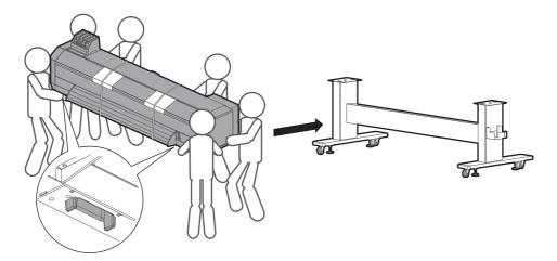
[2] Use the wing bolts (×8) and attach the printer to the stand.
