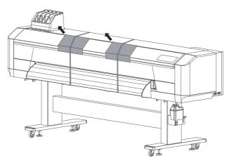
[2] Open the front cover and remove the protective tape from the maintenance cover.
