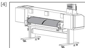
From the rear side of the printer, insert the front edge of the media into the media slot.
