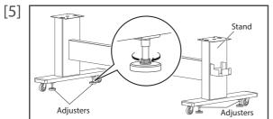
Turn the leveling adjusters (×4) as shown on the left until the stand does not move.
