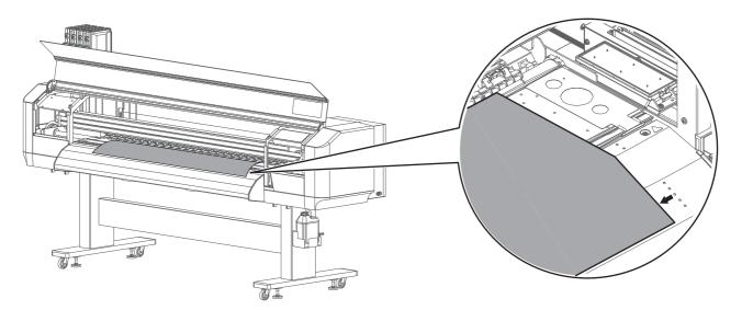
[8] If needed, use a slide lock lever on the pressure rollers to individually cancel or reduce the pressure.
