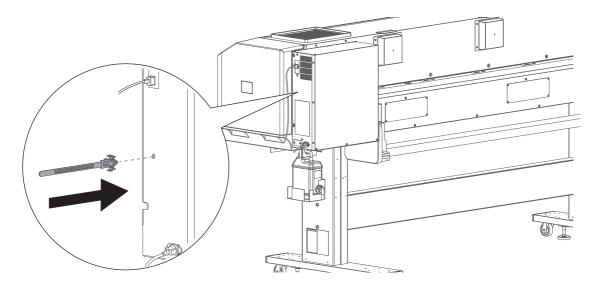
[4] Use the cable tie to secure the Ethernet cable to the printer.
