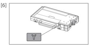
Apply an ink color label onto the outside of the case.
